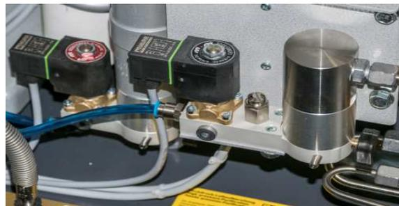
B-DRAIN Automatic condensate drain system
